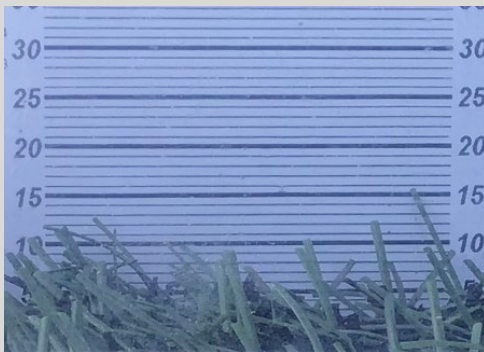
Figure 5 - Free pile height in Location 2 (far side penalty)
