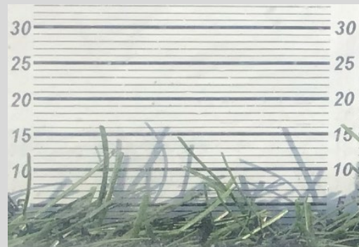
Figure 6 - Free pile height in Location 5 (near side penalty)
